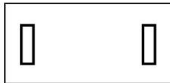
Floor plan of the initial state with two eccentrically braced building halves (above) and floor plan of the retrofitted state with a centrally braced building (below).
