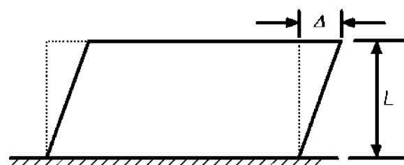
FIG. 10-5. Story Drift in Shear Wall where Shear Dominates Inelastic Response
